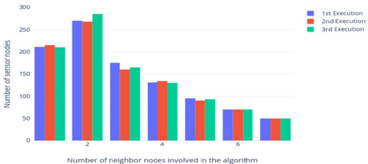
Figure 8: Number of neighbor nodes involved in the routing algorithm towards the gateway with N = 1000 , G = 10 , and r = 100 \text{ m}
