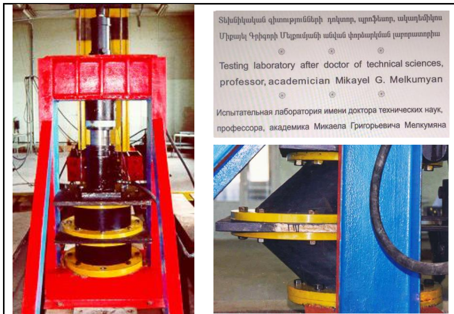
Fig. 13. Facilities in the laboratory named after the author of this paper and designed by him for testing of different types of the seismic isolation laminated rubber-steel bearings
