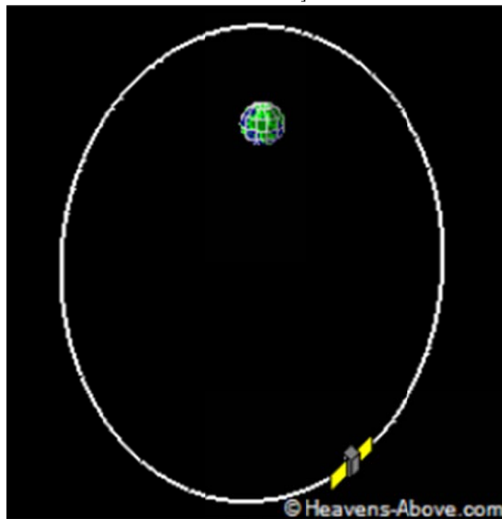
Figure 3 The orbital view of XMM satellite which has eccentricity value of 0.5960958 [Source: https://www.heavens-above.com/ ]
